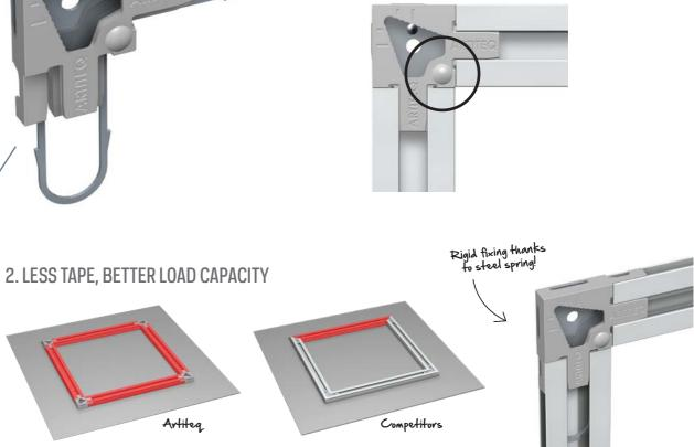
Power Corners enable equal weight distribution because of rigid fixing thanks to steel spring in square-cut profiles instead of mitre-cut profiles.
